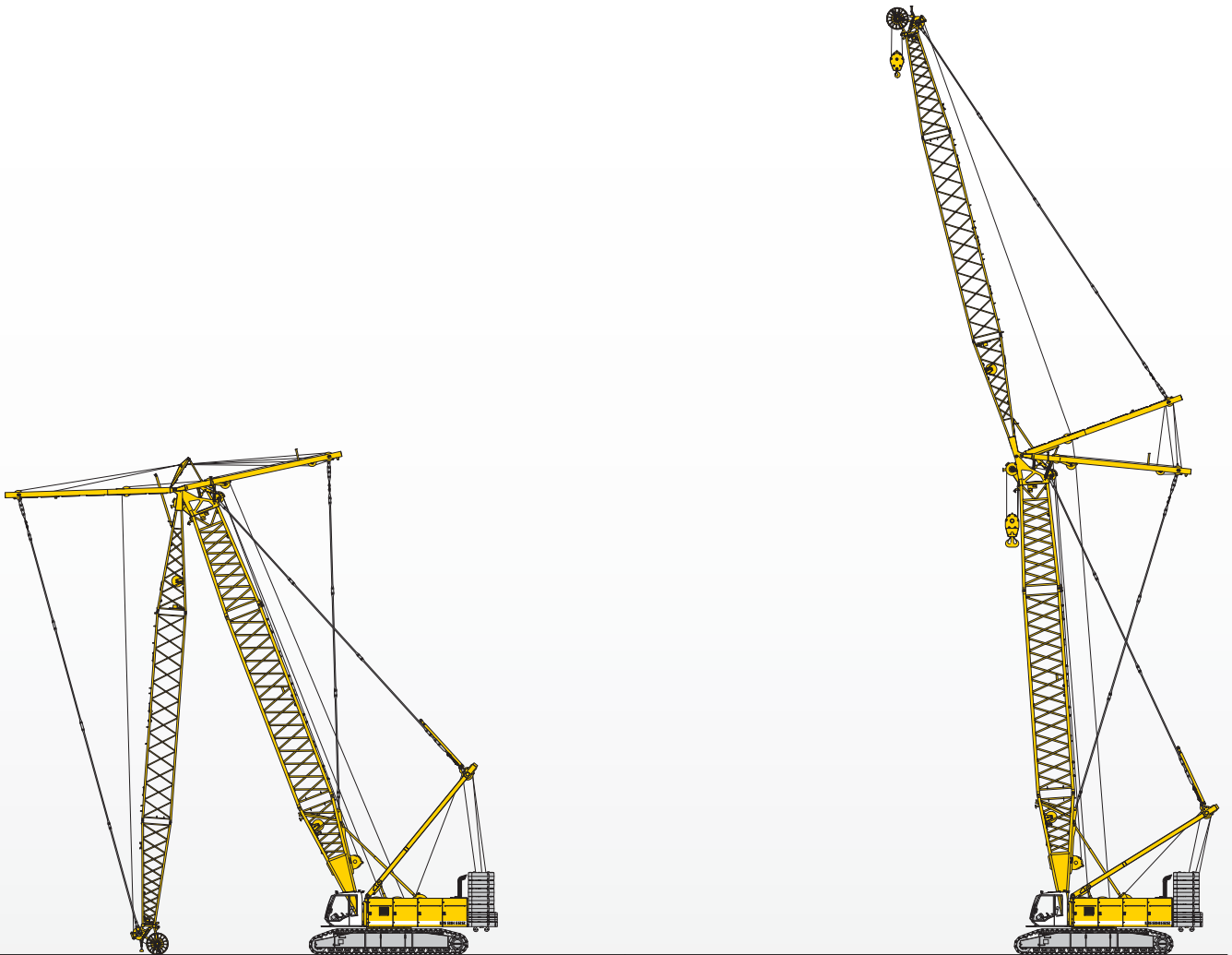
Erecting of main boom and luffing jib
