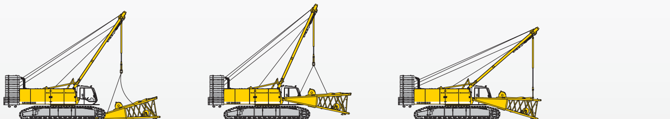
Unloading and assembly of boom foot
